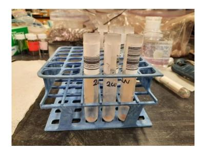
9. Pretreatment of soil samples: Once all samples are weighed out (28 tubes maximum per set), then slowly add 5 mL of water to each tube, put the cap on and make sure they are solidly attaching (preferably use the tape around the cap) and place them on the sample rotator for 24 hours.
