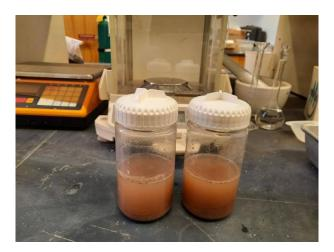
Loosen caps to allow gas to escape, then place bottles in a hot water bath. Heat until bubbling stops (<30 min).
